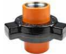
Figure 602 Threaded 6000 PSI CWP Specially Designed Lip Type Elastomer Seal Protects Metal to Metal Sealing Surface and Reduces Line Flow Turbulence
